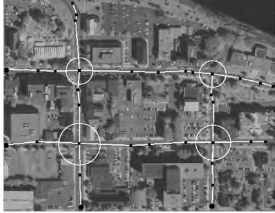
FIGURE 11.9 Topological graph subsampling.
