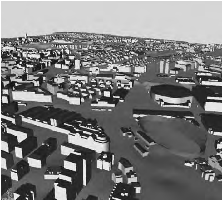
FIGURE 14.4 City model Zürich Oerlikon. Note the modeling of nonplanar surface objects.
