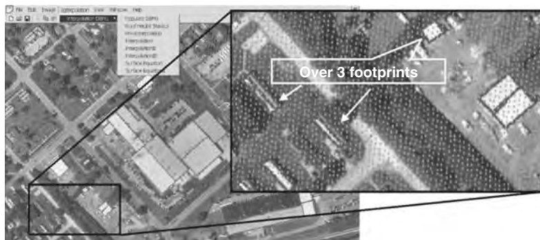
FIGURE 13.13 Human-computer interaction for house interpretation, and the number of LiDAR footprints within a house.
