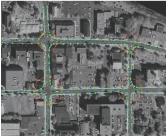
FIGURE 11.11 Final result after the extraction of intersections.
