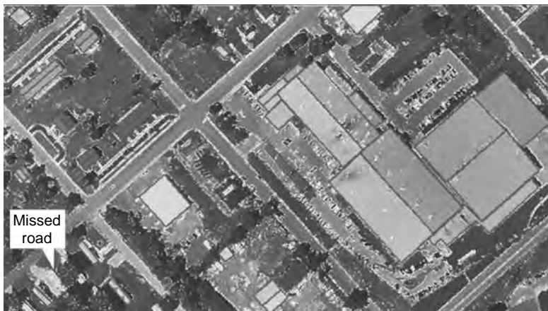
FIGURE 13.8 Building edges detected by human-computer interaction operation.
