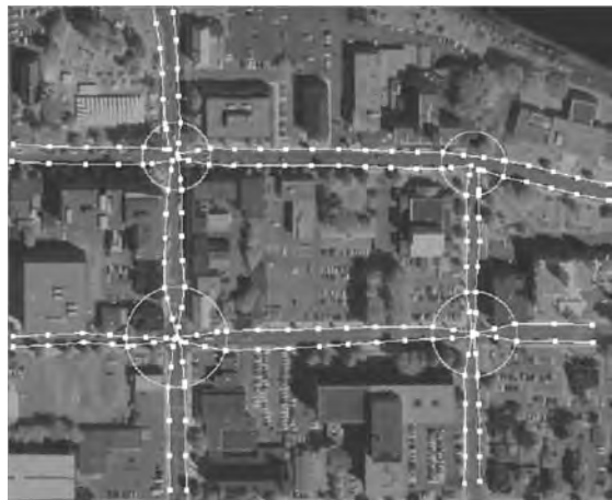
FIGURE 11.10 Intersection initialization after road segment extraction.
