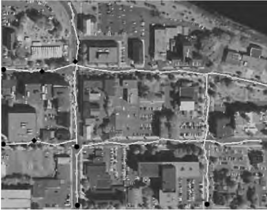
FIGURE 11.7 After the extraction of polylines by the tracking algorithm.
