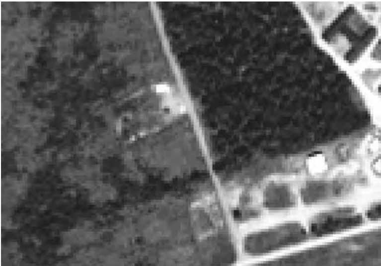
FIGURE 16.7 QuickBird multispectral image of rural scene close to Fredericton (subset, 2.8 m resolution).
